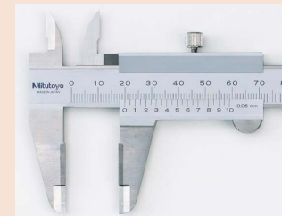
530-320 (Carbide-tipped jaws for outside measurement)
