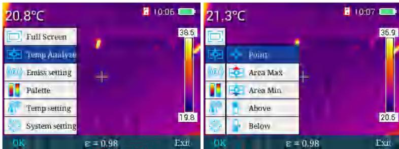
Test temperature of central point in “point” analysis mode, as shown below.
