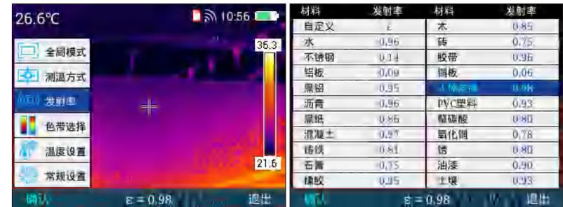
It is also allowed for user-defined emissivity value. In emissivity mode, go to custom mode, select “confirm” key, and then press “+” and “-” keys to customize emissivity value ranging from 0.01 to 1.00. Press “exit” key to back to main menu.
