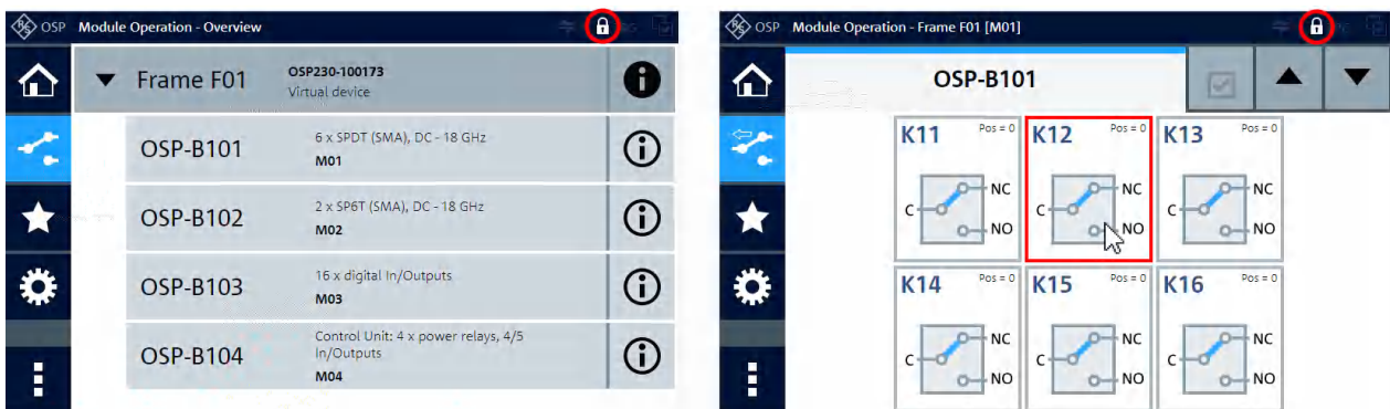
Figure 5-21: Module Operation dialog of a switch unit and of one module in lock mode
