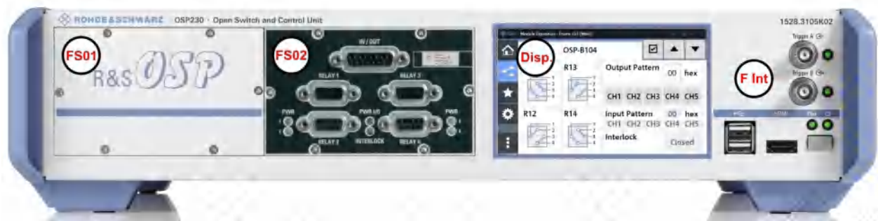
Figure 2-4: Front view of the R&S OSP230 (2HU)
