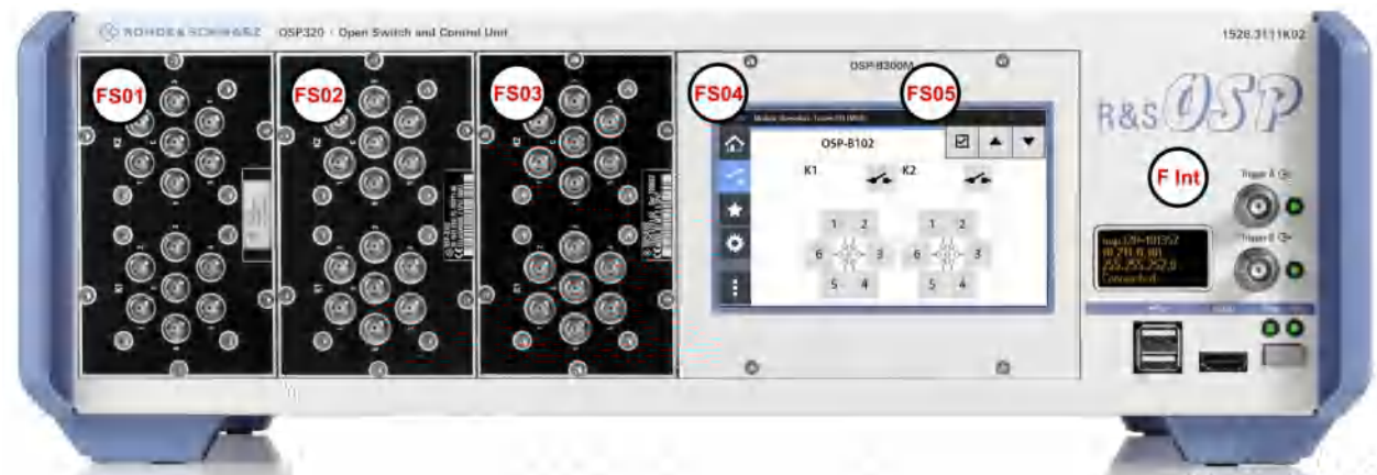
Figure 2-5: Front view of the R&S OSP320 (3HU)
