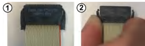
Figure 2-24: To attach or release the cable, press the latches on the sides of its connector
