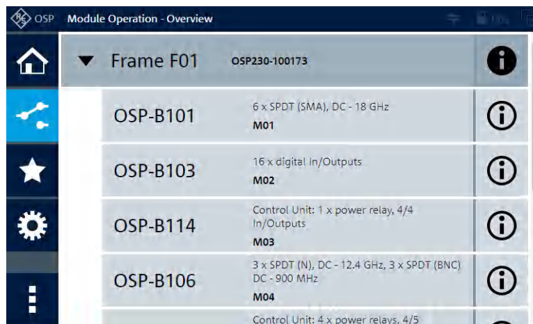
Figure 2-2: The module operation dialog, here with a single switch unit and 5 modules
