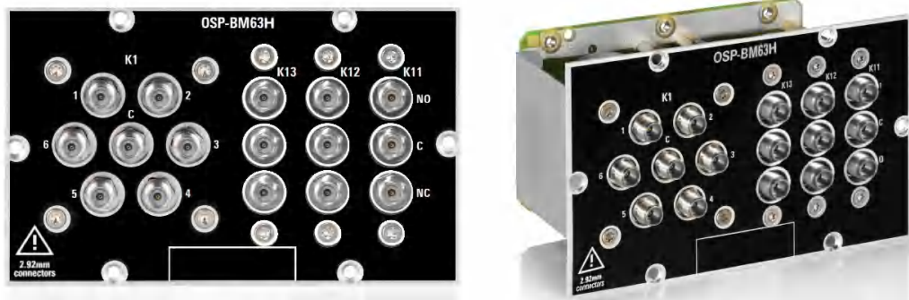
Figure 3-8: R&S OSP-BM6xH (here with 1 SP6T + 3 SPDT relays)
