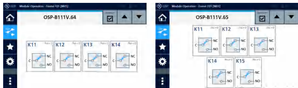
Figure 3-50: Representation of the module on the control screen, here with 4 or 5 SPDT relays
