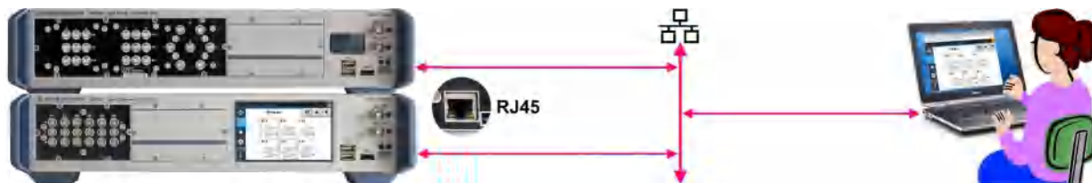
Figure 2-14: Manual remote operation via "WebGUI" and LAN
