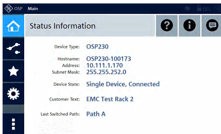
Figure 2-17: Main menu of the graphical user interface ("WebGUI"), here in the recommended Chrome browser
