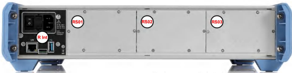
Figure 2-9: Rear view of the R&S OSP220 (2HU)
