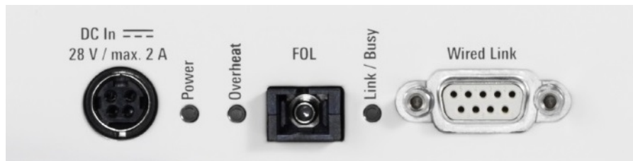
Figure 3-139: Connectors and LEDs on the rear panel of the R&S OSP-B200S2
