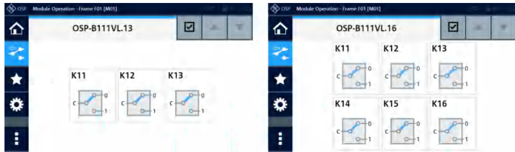
Figure 3-53: Representation of the module on the control screen, with 3 or 6 SPDT relays
