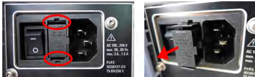
Figure 12-1: Removing the fuse holder (holes to unlock marked red)
