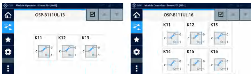
Figure 3-48: Representation of the module on the control screen, with 3 or 6 SPDT relays
