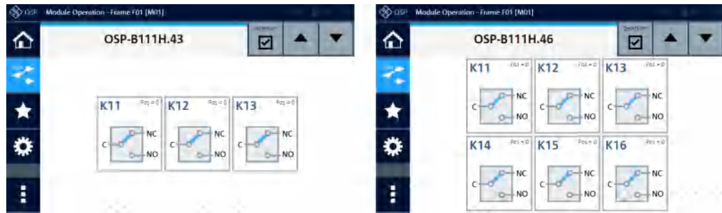
Figure 3-44: Representation of the module on the control screen, with 3 or 6 SPDT relays
