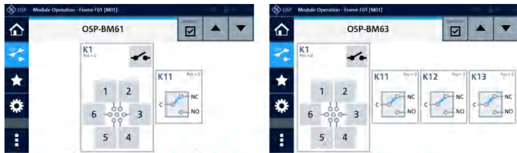
Figure 3-6: Representation of the module on the control screen (left: 1 SPDT, right: 3 SPDT)
