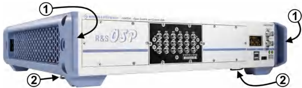
Figure 2-1: Handles (1) for lifting and carrying the R&S OSP. Underneath: foldable feet (2)
