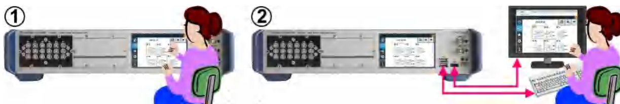
Figure 2-13: Operation by integrated touchscreen (1) or by external USB / HDMI devices (2)
