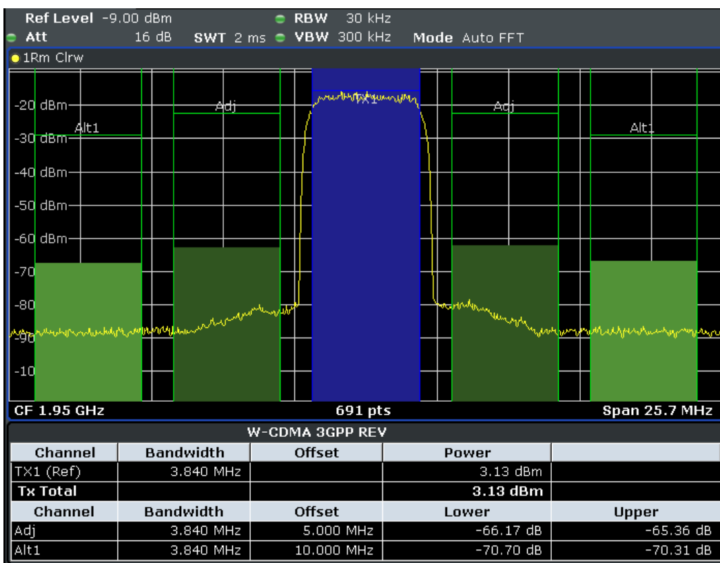
Figure 6-33: Measuring the relative adjacent channel power on a W-CDMA uplink signal
