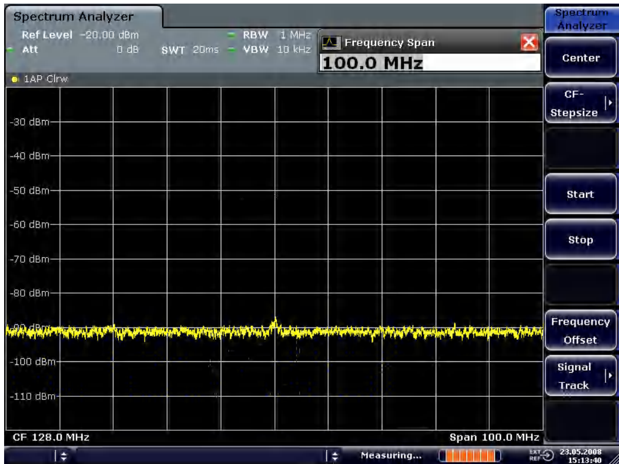
Figure 6-27: RF sine wave signal with low S/N ratio if a smaller video bandwidth is selected.
