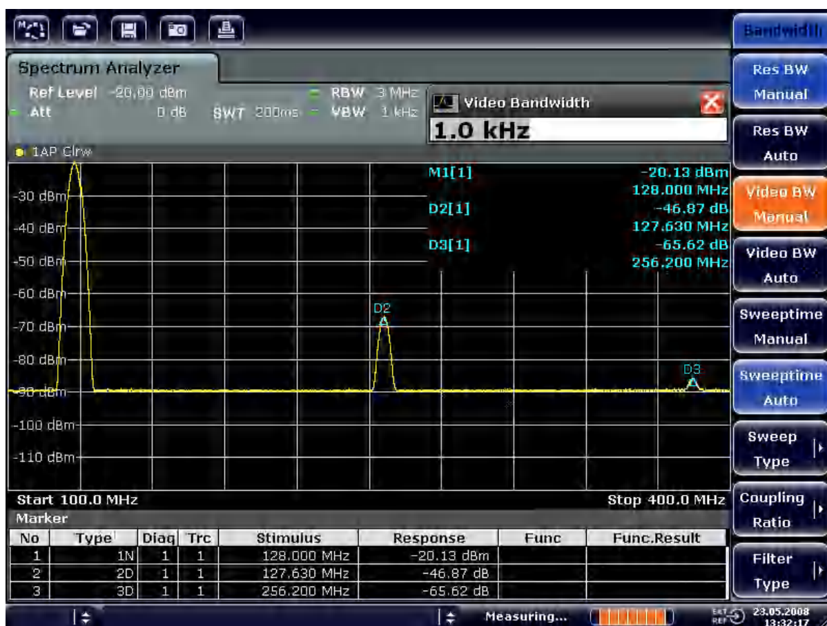
Figure 3-10: Suppression of noise during harmonics measurement by reducing video bandwidth
