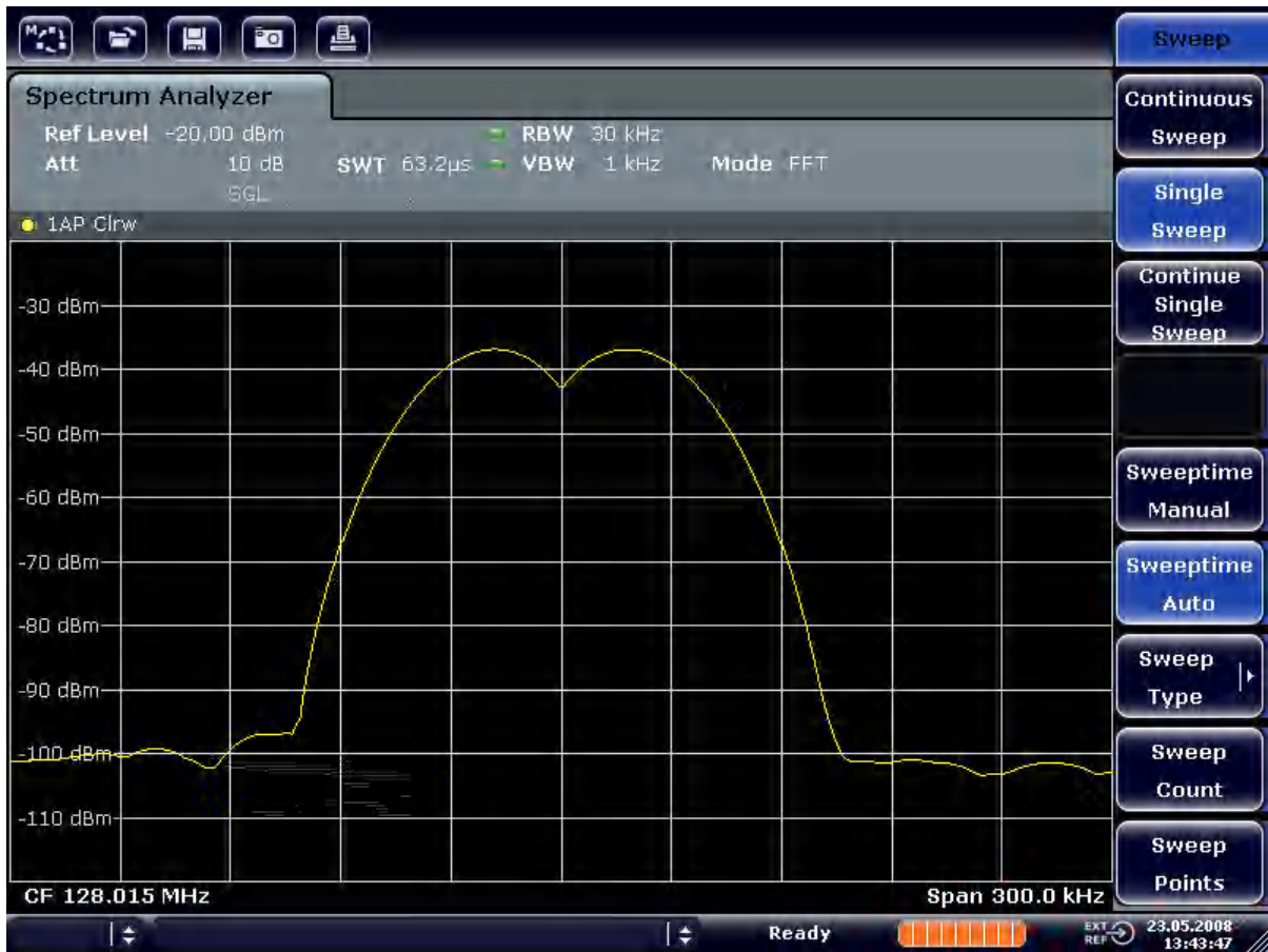
Figure 3-11: Measurement of two equally-leveled RF sinusoidal signals with the resolution bandwidth which corresponds to the frequency spacing of the signals
