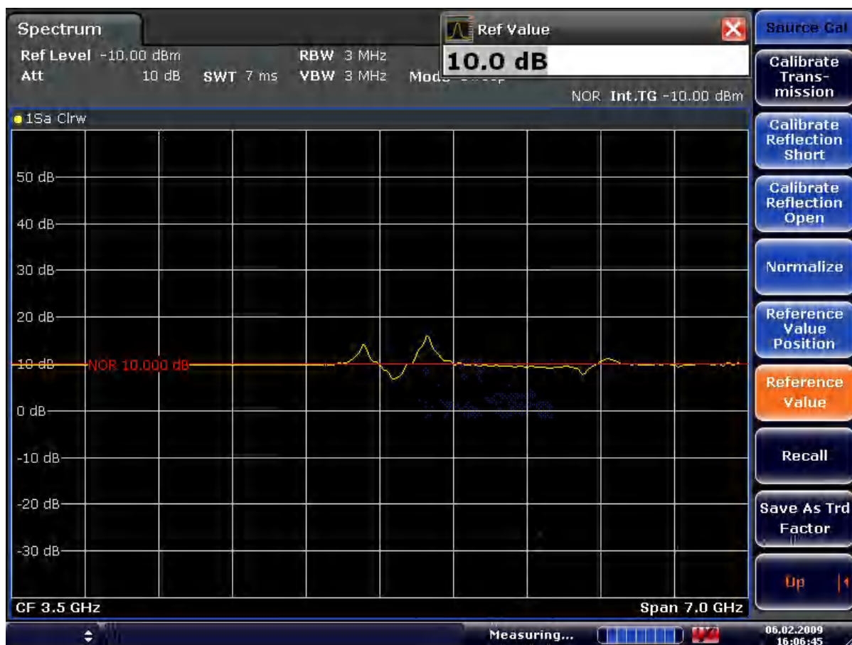
Figure 8-7: Measurement with Reference Value: +10dB and Reference Value Position = 50%
