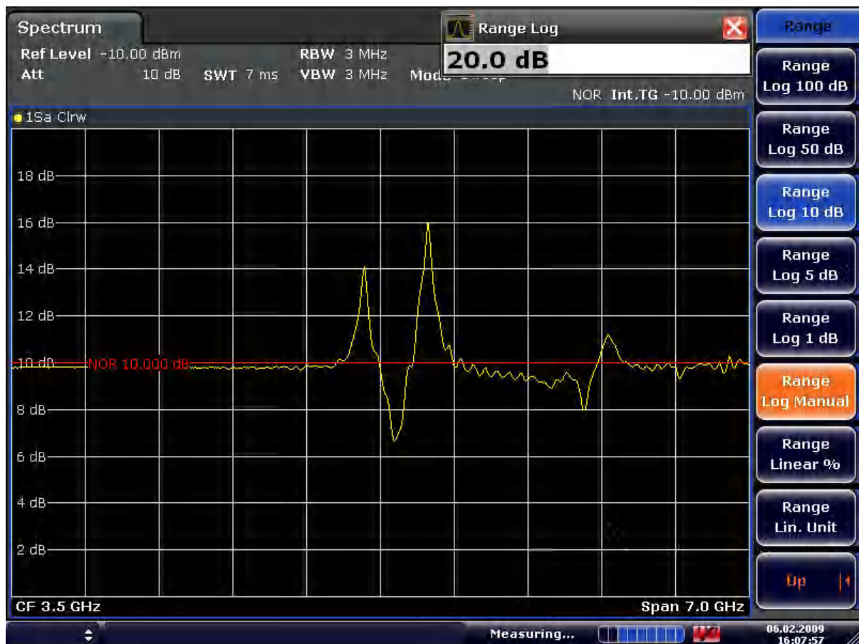
Figure 8-8: Measurement of a 10-dB attenuator pad with 2dB/Div
