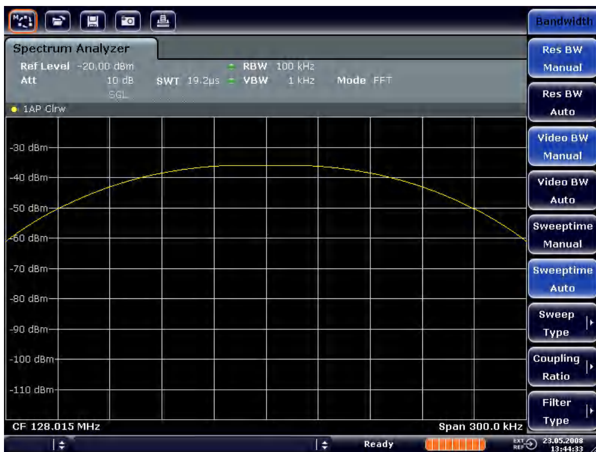
Figure 3-12: Measurement of two equally-leveled RF sinusoidal signals with a resolution bandwidth which is larger than their frequency spacing
