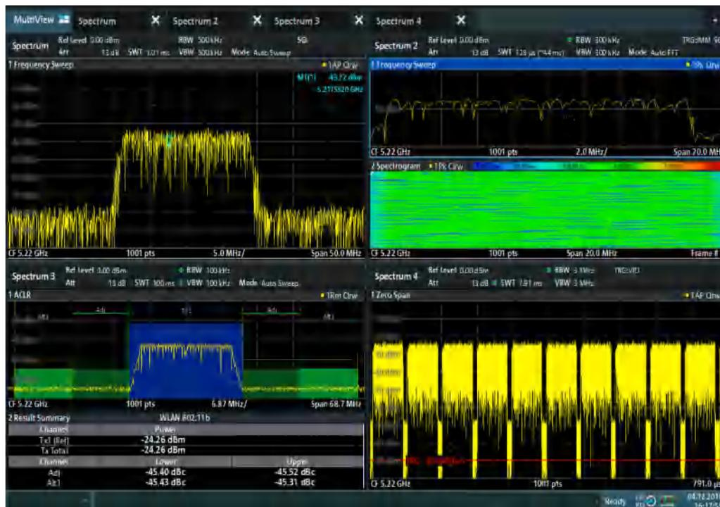
Screenshot of the R&S®FPL1000 with MultiView. The sequencer consecutively performs a spectrum measurement, an adjacent channel power measurement, a time domain measurement (zero span) and a spectrogram measurement. The results are displayed clearly and simultaneously. The toolbar on the left allows fast access to the most common menu functions. Different measurements can be activated with the tabs at the top.
