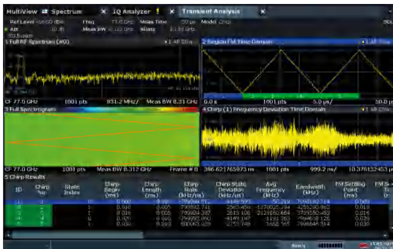
Analysis of an FMCW signal with the R&S®FSW-K60C option and 8.3 GHz analysis bandwidth
