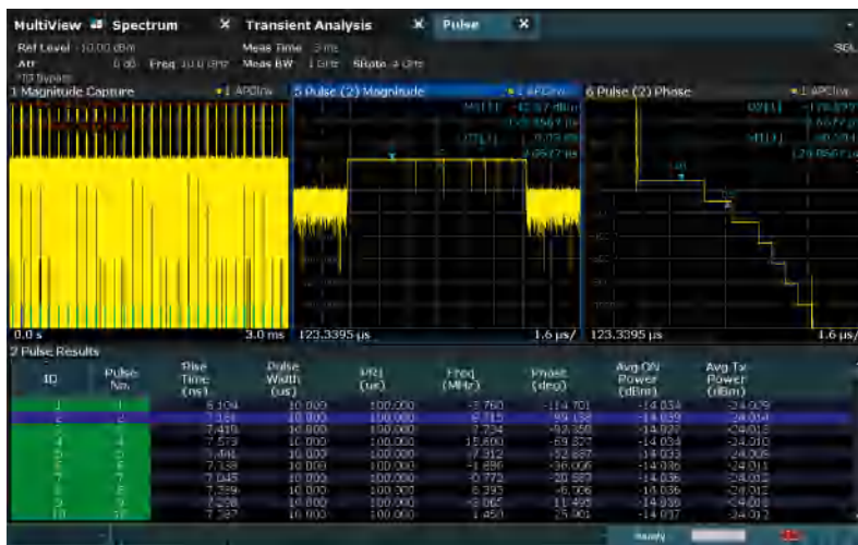
Equipped with the R&S®FSW-K6 pulse measurements option, the R&S®FSW delivers pulse parameters at the touch of a button
