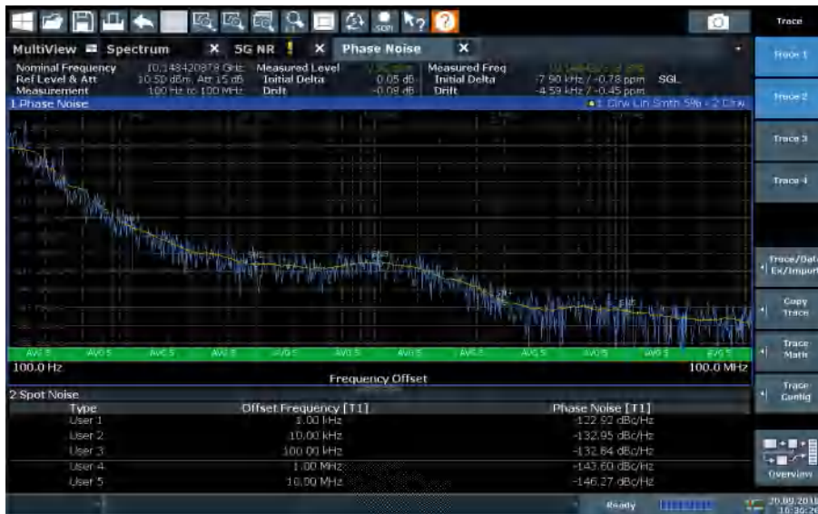
Phase noise at 10 kHz offset from a 10 GHz carrier: typ. -133 dBc (1 Hz)
