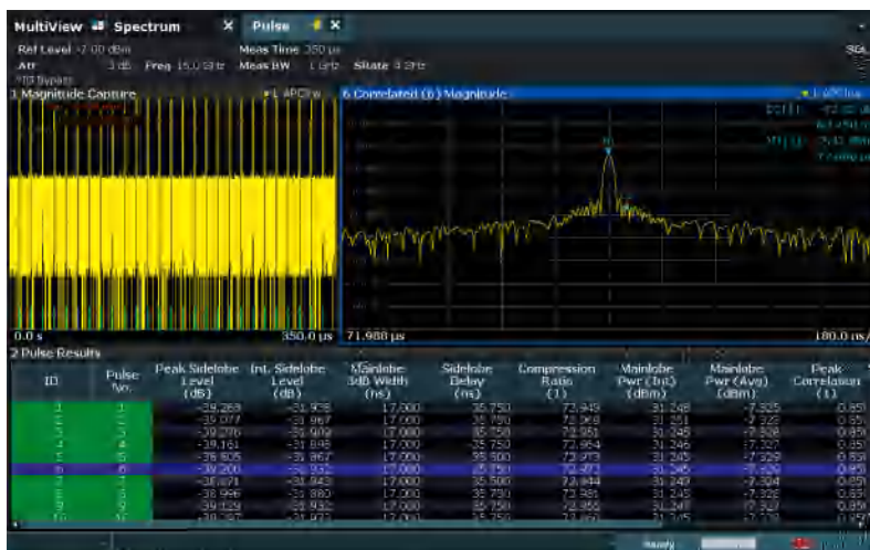
Pulse compression parameters and correlated magnitude display of a chirped pulse are shown with the R&S®FSW-K6S option
