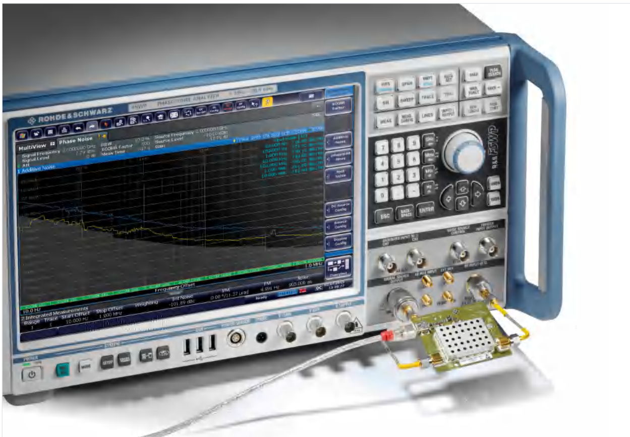
Typical setup for measuring the residual phase noise of an amplifier and displaying the resulting trace
