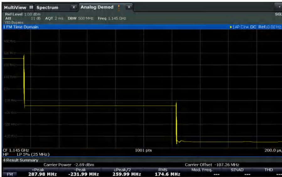
Wideband frequency analysis of a synthesizer. The trace shows frequency versus time. This enables the user to measure switching times and check frequencies.
