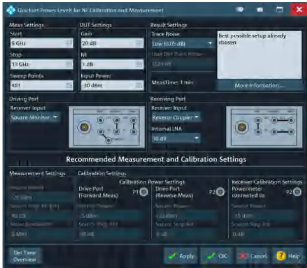
Quickset dialog for interactive and semi-automatic configuration of optimal test parameters and R&S ZNA hardware.
