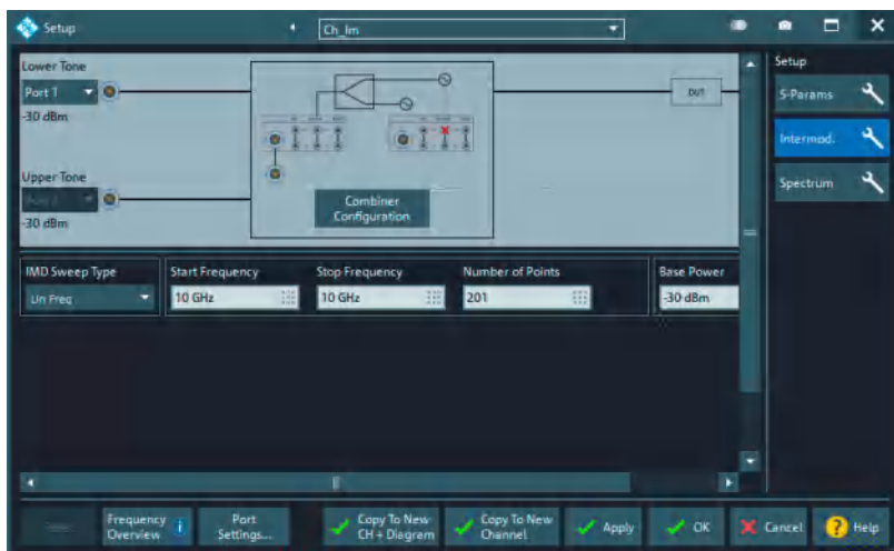
Power calibration GUI for an amplifier intermodulation measurement.
