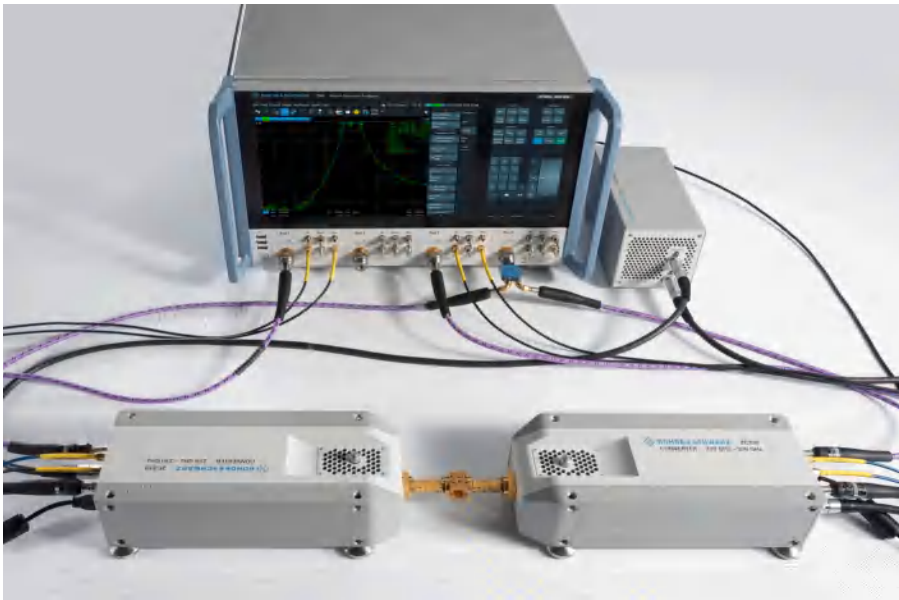
Setup for mmWave measurements with an R&S®ZNA43 and two R&S®ZC330 mmWave converters WM-864.
