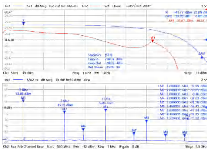
R&S®ZNA-K1 spectrum analyzer option: amplifier magnitude and phase compression measurement (at 1 GHz, top), and corresponding harmonic and spurious spectrum.
