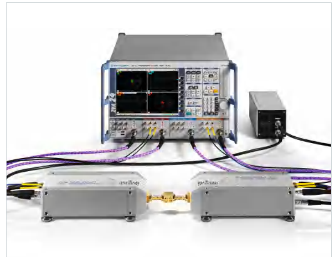
Setup for a two-port measurement in WM-864 band with an R&S®ZVA24 vector network analyzer.
