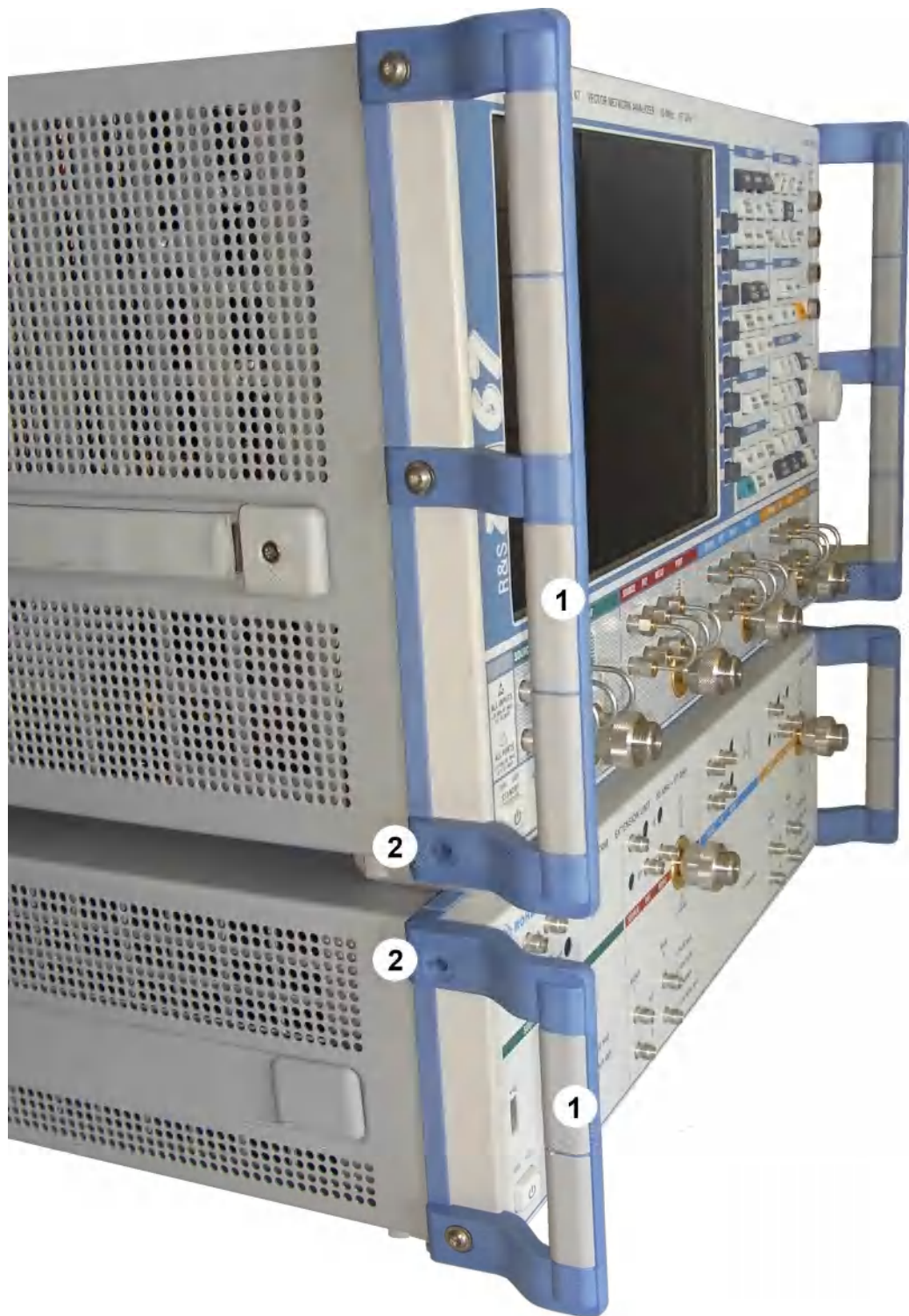
Figure 3-3: R&S ZVA67 stacked on top of R&S ZVAX-TRM, units not yet fixed by adapters and screws
