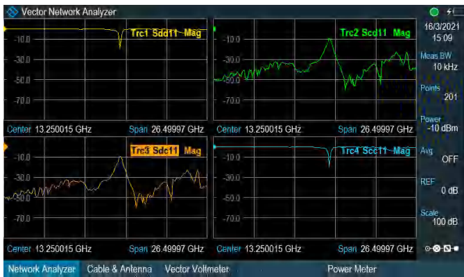
R&S®ZNH-K47 mixed mode measurement.
