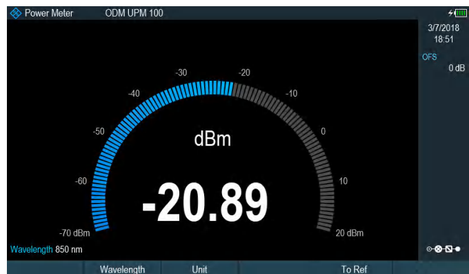
Optical power measurement with optical power sensor.
