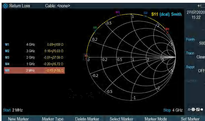
Return loss measurement – Smith chart display.
