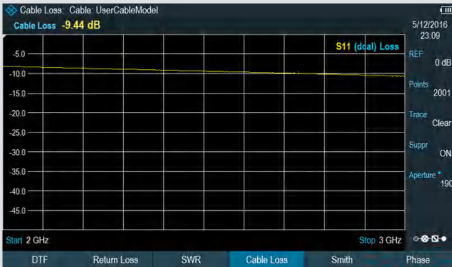
One-port cable loss measurement
