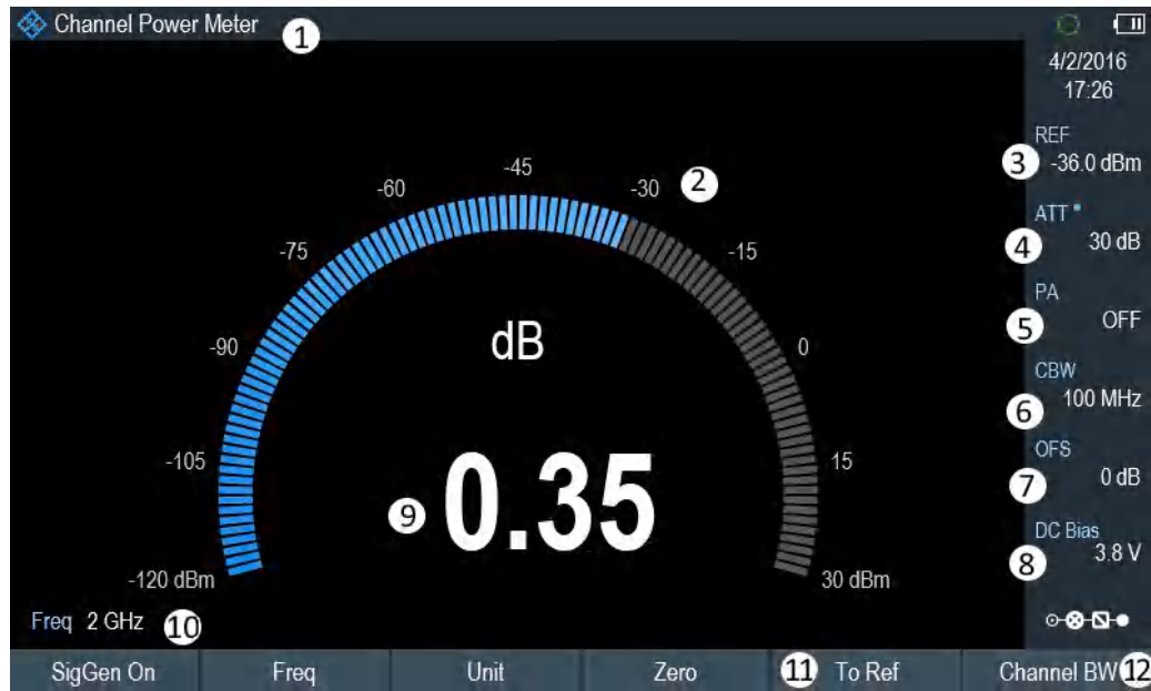
Figure 10-1: Internal power meter measurement
