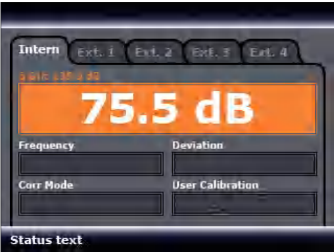
Automatic detection and display of external step attenuators.
