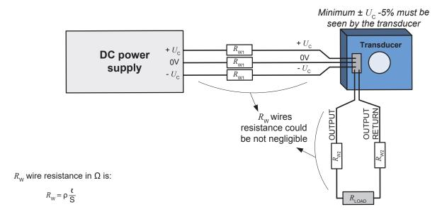
S: Cross section of wire in m<sup>2</sup>
