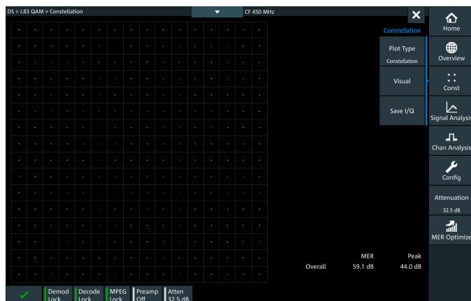
J.83 constellation diagram with 256QAM
