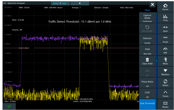
OFDMA upstream signal with traffic detect threshold set
