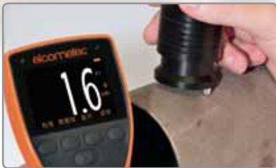
整体式分体式探头测得的粗糙度高达500 \mu\text{m} (20mils)
