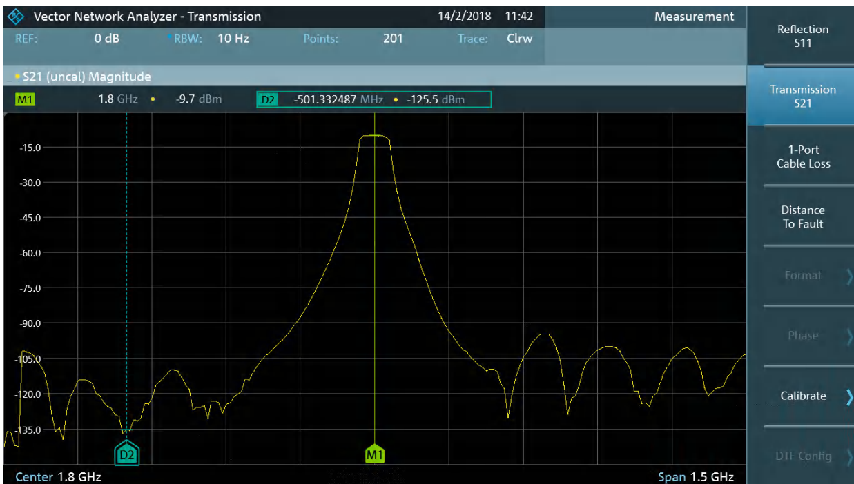
R&S®FPC1500 S_{21} 标量传输测量，配备 R&S®FPC-K42 选项
