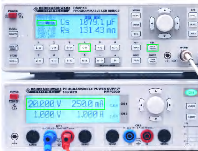
Fig. 7.5: Activate external BIAS preload
