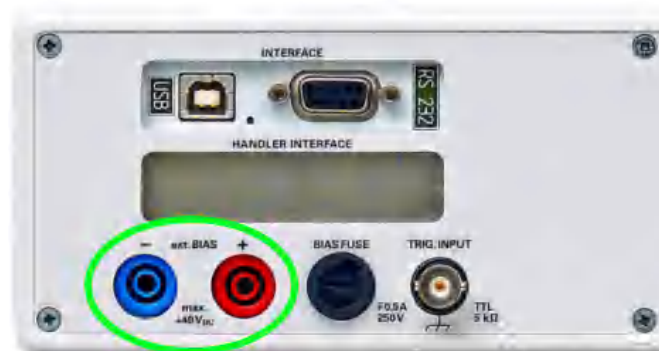
Fig. 7.4: Connectors for external BIAS preload
