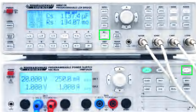
Fig. 7.6: Activate external BIAS preload
