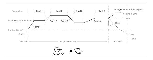
Advanced functions include 8-segment Ramp/Dwell, USB interface, and Analog DC output capability
