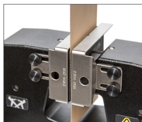
Jaw Face Shields reduce pinch hazards and have useful specimen alignment features.
