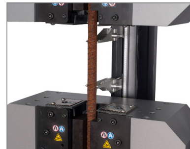
Rebar Test with AutoX750 on a 1500KPX Hydraulic Frame
