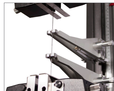
Carbon Fiber Tow in Pneumatic Side-Action Grips with AutoX750
