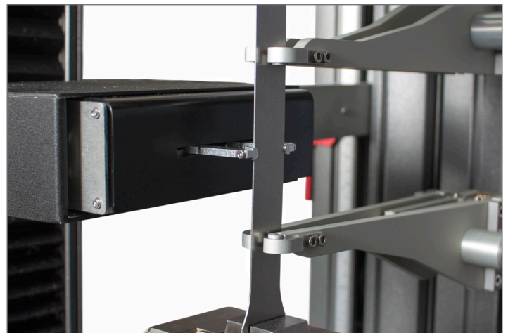
AutoXBiax Automatically Centers in Gauge Length
