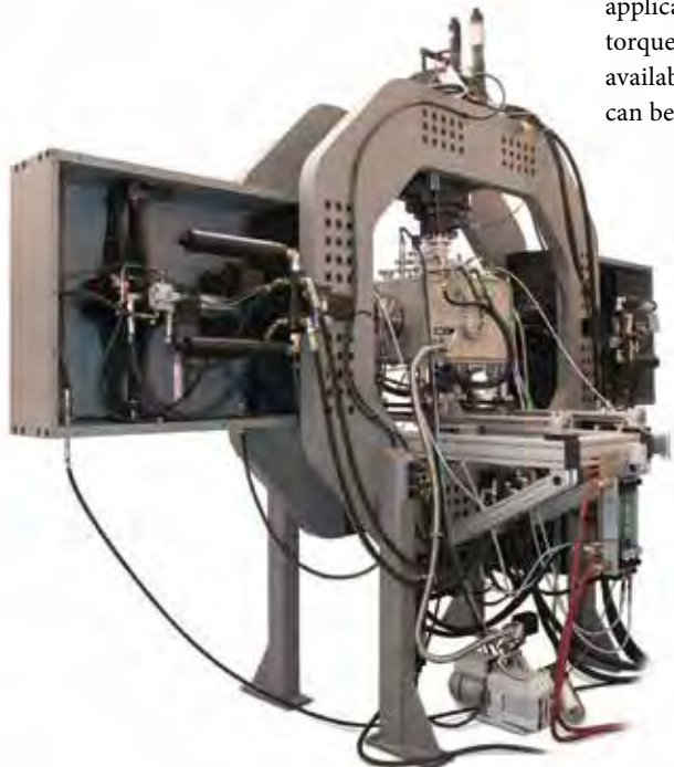
Rear side of MTS Planar Biaxial System with torsion. The torsion actuator is visible in the left side of the picture about midway from top to bottom. In addition, a high temperature vacuum chamber is seen in the test area. There are rails mounted to the frame to locate the vacuum chamber and allow easy installation and removal.
