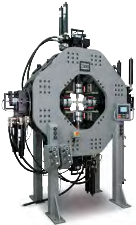
MTS Planar Biaxial 100 kN System with small compact frame design. Hydraulic grips are common and the grip controls are mounted on the left front leg. The structure with the red pads mounted to the frame between the silver colored hydraulic grips is the passive restraint system.
