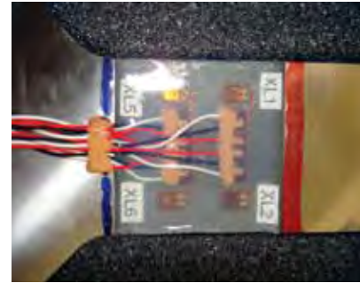
Instrumented specimen showing 4 strain gages on this side of one arm. There are 4 more strain gages on the other side of the arm, or 8 gages per arm with a total of 32 gages.
