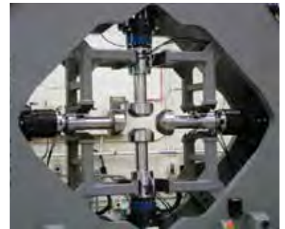
MTS Planar Biaxial 100 kN System with large test area designed to provide space for an environmental chamber. Visible in this photo is the passive restraint system and MTS extension rods and hydraulic grips to fit inside the chamber (chamber not in picture). The grips are specially modified to remove extraneous material allowing them to get closer together and grip smaller specimens with shorter arms with no decrease in grip capacity.
