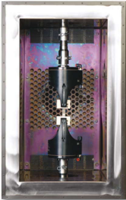
Load extension kit and pneumatic grips in an environmental chamber
