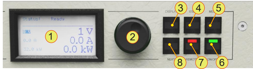
Fig. 5 Controls for the optional HMI (or the RCU).
