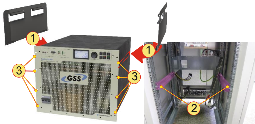
Fig. 9 Prinziple picture to show the procedure of the TopCon device installation.
