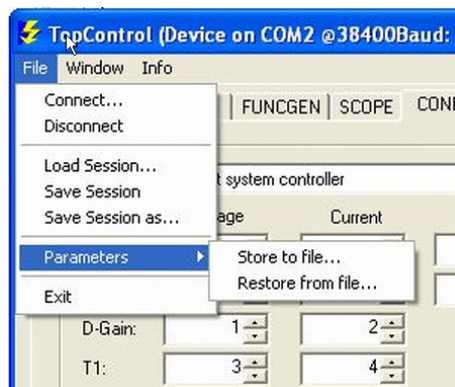
Fig. 28 Using TopControl to save/load config and protect parameters
