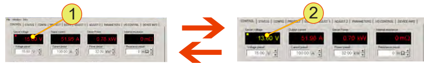
Fig. 22 Indication of the sense actual values. Example voltage value in normal state -1- and actual value is not reached -2-.
