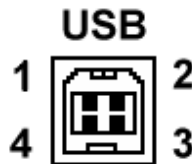
Figure 3-2: USB Connector pin orientation
