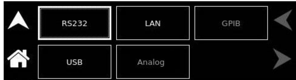
Figure 3-103: Control Interface Menu Screen with Analog disabled
