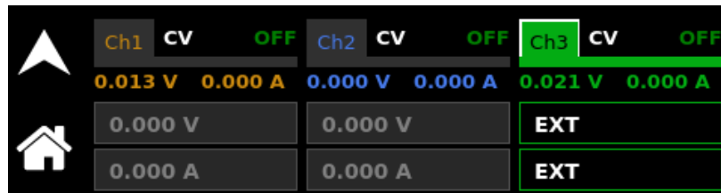
Figure 3-25: Output Voltage and current as EXT Reference Mode for Channel 3
