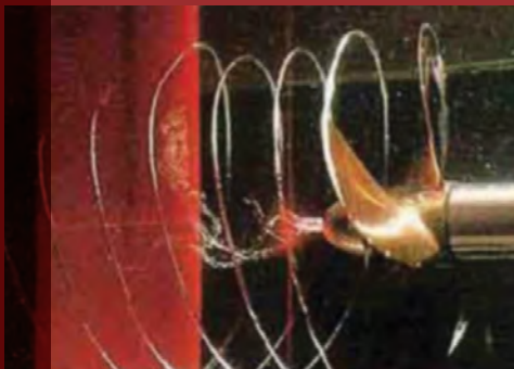
3D LDV System for the measurement of flow behind propeller, INSEAN, Italy
