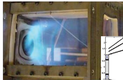
PDPA measurement of a Lean Low NOx Aircraft Combustible spray with SMD result, Georgia Institute of Technology, USA
