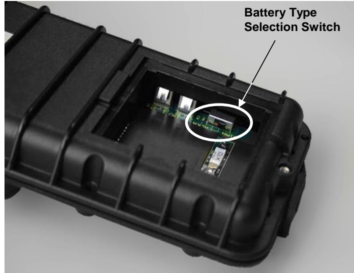
Figure 2-1 Location of Battery-Type Selection Switch
