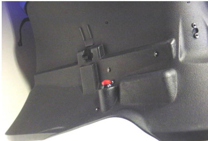
Figure 8 Red Hold Switch Location
