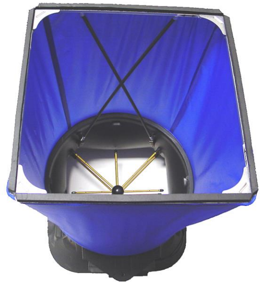
Figure 3 Installing the Support Poles on a 16 in × 16 in (406 mm × 406 mm) Hood
