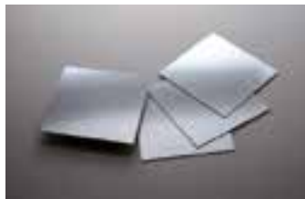
Passivation layers: Cr/Zn/Fe
