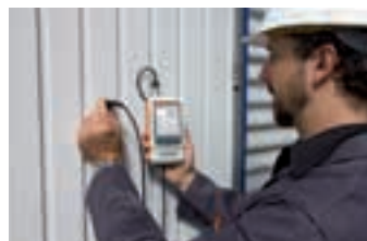
Measurement of a paint coating on steel
