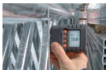
Measurement of anodizing on aluminum frames for building cladding
