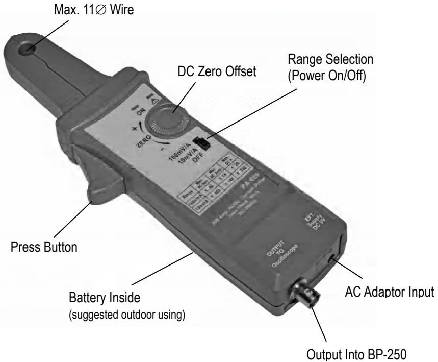
Figure 1: shows the controls and indicators on the PA-629 current probe.
