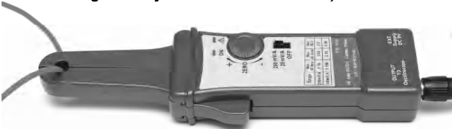
Figure 2: Connecting the PA-659 current probe.
