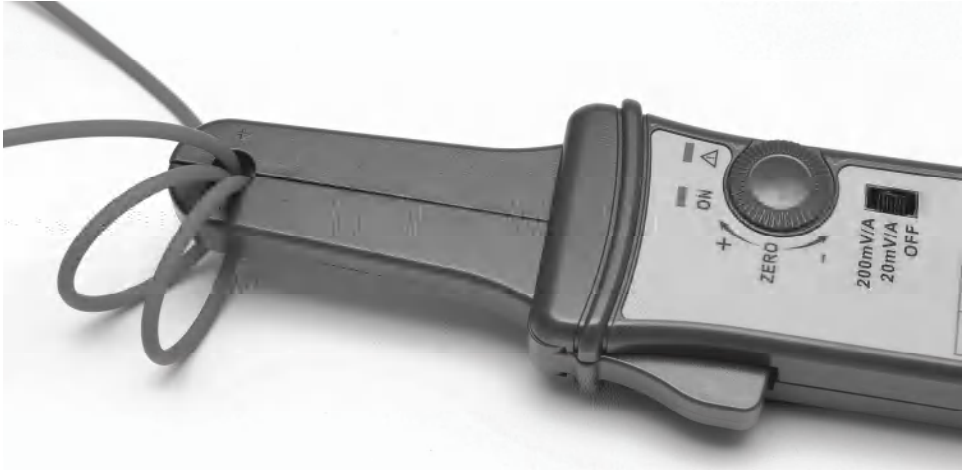
Figure 4: Increasing the sensitivity
