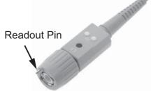
The CP-3501R/Pro is compatible with readout function oscilloscopes that automatically detect and display the attenuation factor of the probe.
