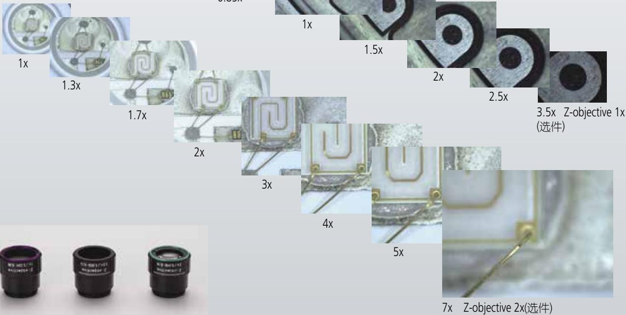
Z-objective 1× (选件)    Z-objective 1.5× (标配)    Z-objective 2× (选件)
