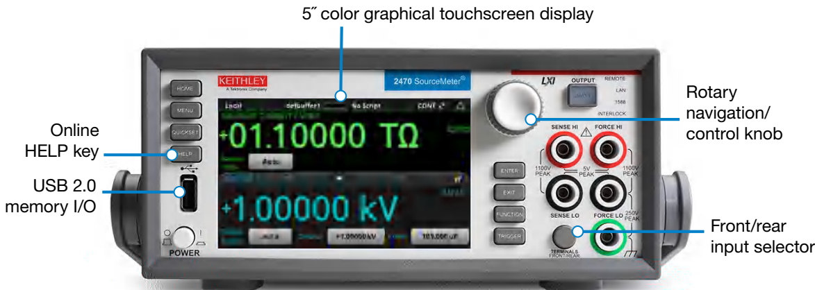
2470 front panel with high-resolution, capacitive touchscreen.
