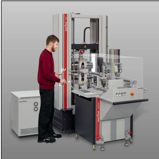
roboTest L robotic testing system for metals
