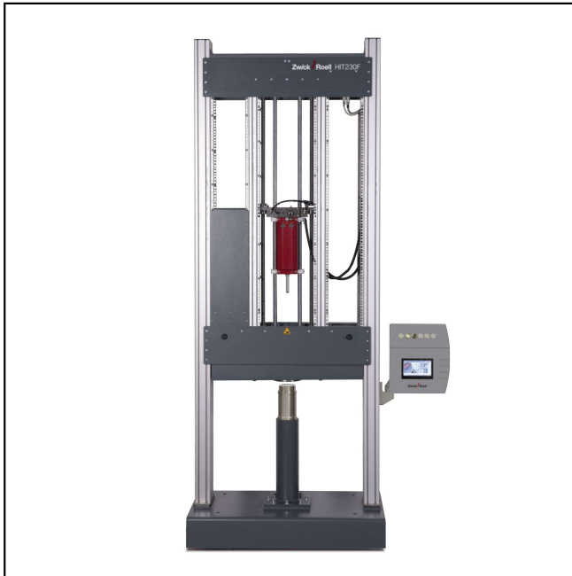
Amsler HIT230F, multiaxial puncture test
