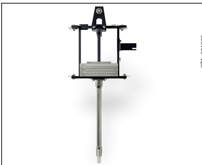
Mass carriage with single masses and Impactor
