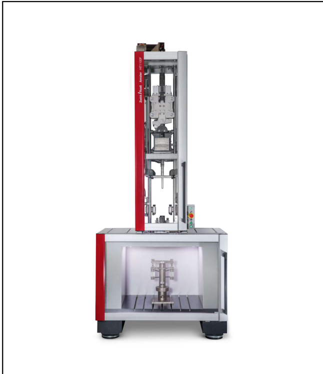
Amsler HIT1100F, multiaxial impact test
