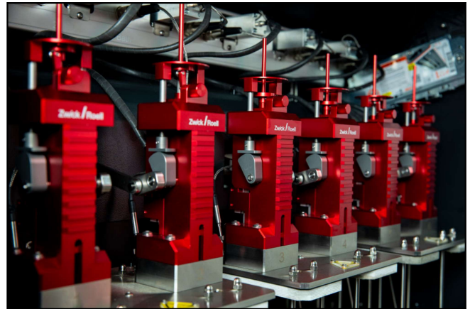
Test station with high precision Digital Displacement Measurement
