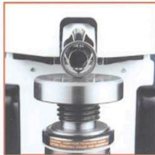
Measuring of the inner contact surface of a bearing's outer ring with 23 mm diameter
