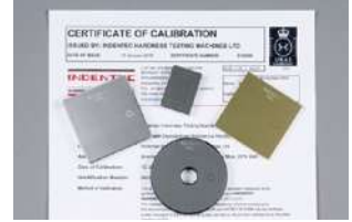
Hardness comparison plate with certificate
