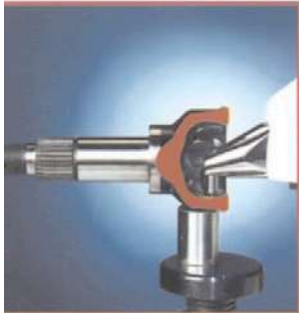
Measuring the inner contact surface
