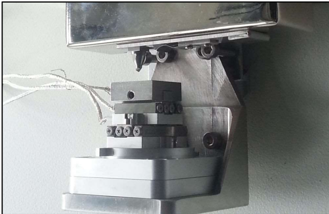
Rotation stage enables rotation around the indenter axis in the X-Y direction
