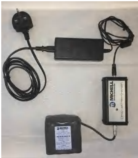
Figure 37 Spare Battery Charging
