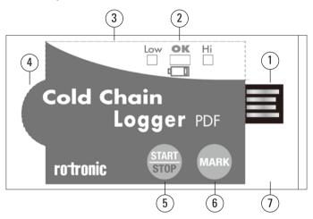
① USB2.0 plug & play connector. USB driver is not required.
