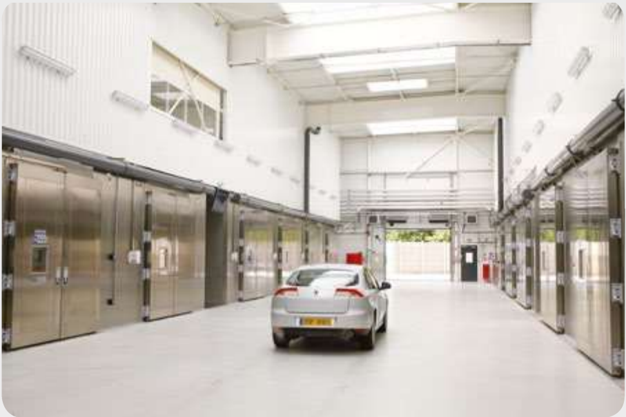
44. Airbag test chamber equipped with a high speed opening and closing door system for quick deployment (7 seconds approx.) of the specimen on a dedicated trolley. 45. Walk-in climatic chambers for corrosion tests on complete vehicles turned-on.
