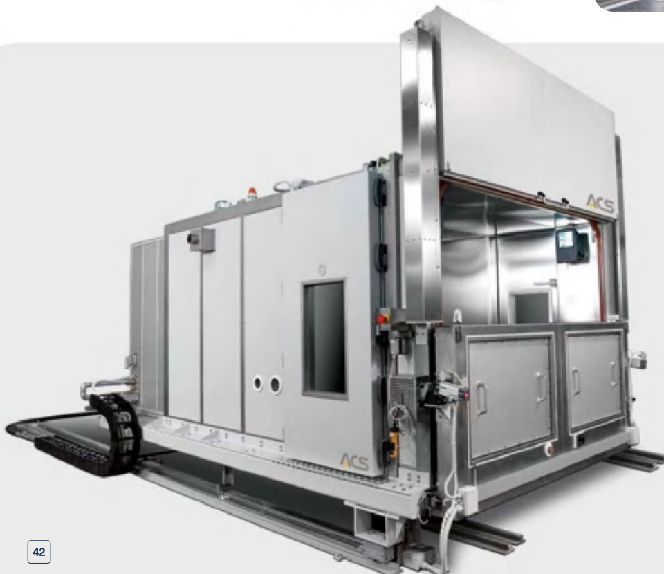
40. Walk-in climatic chamber for thermal transmittance tests on walls materials, domestic doors and windows.
